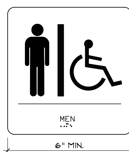
9 A.D.A. ACCESSIBLE TOILET SIGN DETAIL 1/2" = 1'-0" 10440aac
