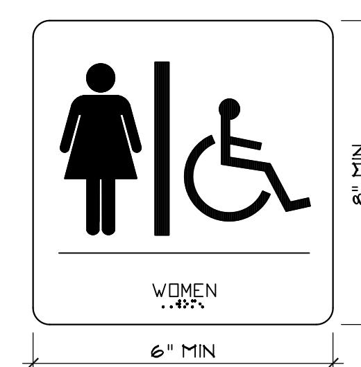
9 A.D.A. ACCESSIBLE TOILET SIGN DETAIL 1/2" = 1'-0" 10440aac
