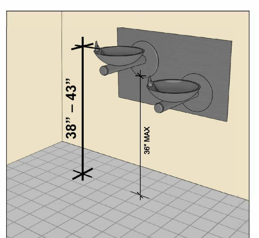
Provisions for wheelchair accessible units require access for a forward approach and address spouts, water flow, and operable parts. Units can be wall mounted or free-standing.
