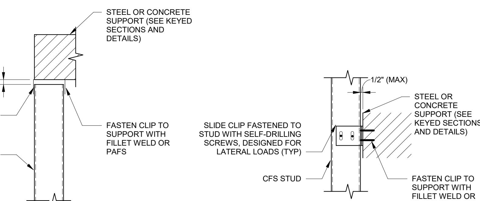
TYPICAL VERTICAL DEFLECTION STUD CONNECTIONS - SECTION
