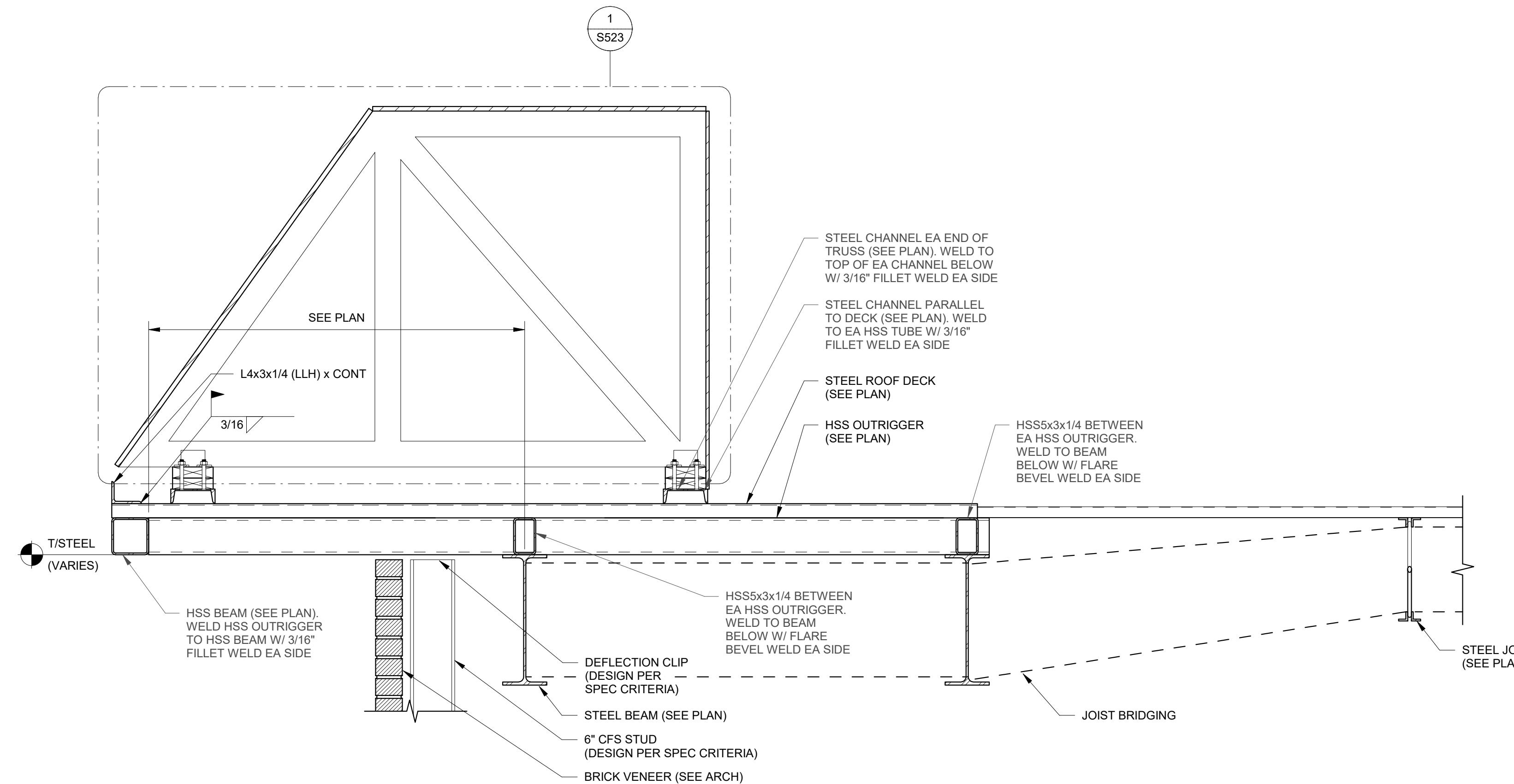
OVERBUILT TRUSS AT DECK BEARING - SECTION
